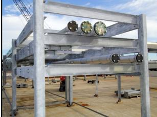
levels utilizing one and a half (1.5) inch to four (4) inch ductile Iron and PVC pipe. The module units were fabricated and assembled in New Hampshire and then shipped out of state. The assembled modules were pressure tested before shipping, and all of the modules were either galvanized or epoxy painted.
